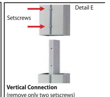
When vertical extrusions are packed in portable cases rather than crates or tubs, they must be broken down into smaller section which then require assembly.
